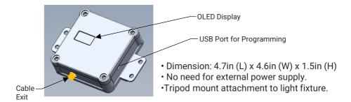
A USB cable establishes communication between a computer and the MLC1 lighting controller. The controller has a Real Time Clock (RTC) and a 1.6 in OLED display for maintaining and displaying accurate time and date.
